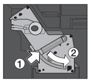
Press the light coloured button under the handle of the brew unit ① and whilst doing so turn the handle in the direction of the arrow ②.
